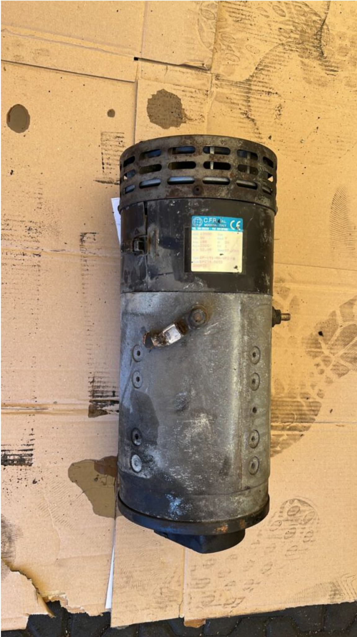
Motor electric stivuator 80V, 188A, 12000W Pret: 1300 € fara TVA Se emite factura
