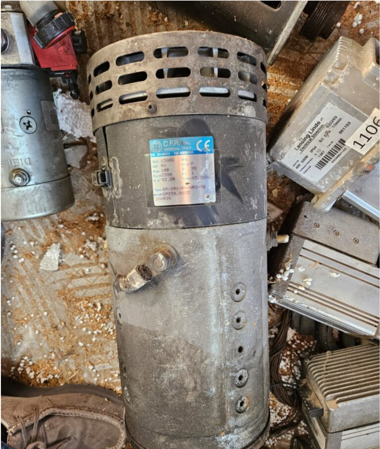
Motor electric stivuator 80V, 188A, 12000W CFR Pret: 1300 € fara TVA Se emite factura
